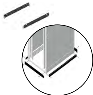
Seal Kit Installation
